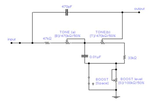
THE TONE CONTROL POT IS A DUAL POT SET UP SO AS TO BOOST MIDS WHEN TREBLE IS CUT.
