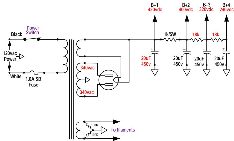
Do not try this at home, kids! This is not a schematic of a working amp but was created to illustrate the similarities. The output section is from the cathode biased Blues Express amp; The voltages shown are high for EL84's.
